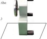
③ Insert the leg as the drawing illustrates. Adjust the height evenly on all three legs. Tighten bolts with allen wrench.
