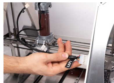
Connect the "LEFT" connector to the Left socket on the machine frame.
