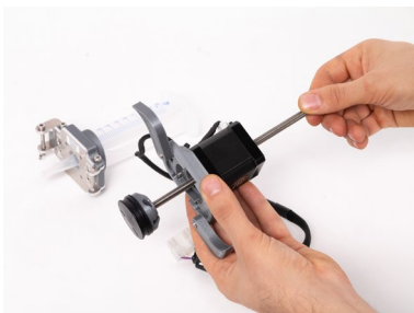
Manually move the piston to the starting position.
