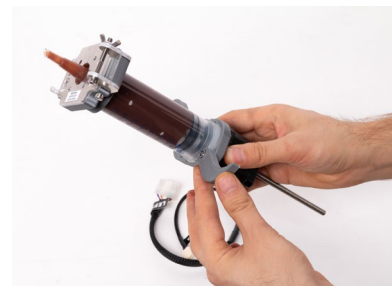
Push the piston inside the syringe and lock the syringe blockade.
